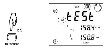
**NOTE:** To avoid measurement errors, do not touch the GroundFlex<sup>®</sup> sensor or the calibration loop during the calibration.
