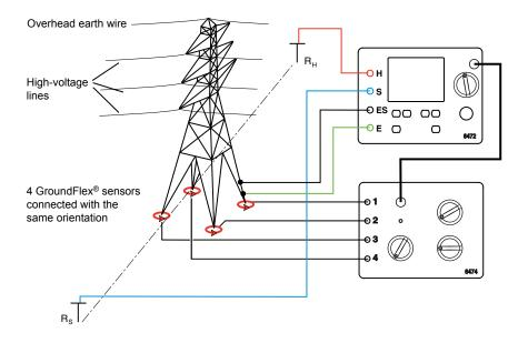
**WARNING:** If the GroundFlex<sup>®</sup> Adapter Model 6474 is connected to the earth tester, the earth potential connected to the terminals **E** (**X**) and **ES** (**Xv**) will also be present at the BNC connectors of the GroundFlex<sup>®</sup> sensors and at the connecting cable between the adapter and tester. Whenever any doubt exists about this earth potential, the user should proceed to a voltage measurement using the **S** (**Y**) and **ES** (**Xv**) terminals of the tester.
