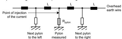
An equivalent diagram of the components forming this circuit is as follows:
