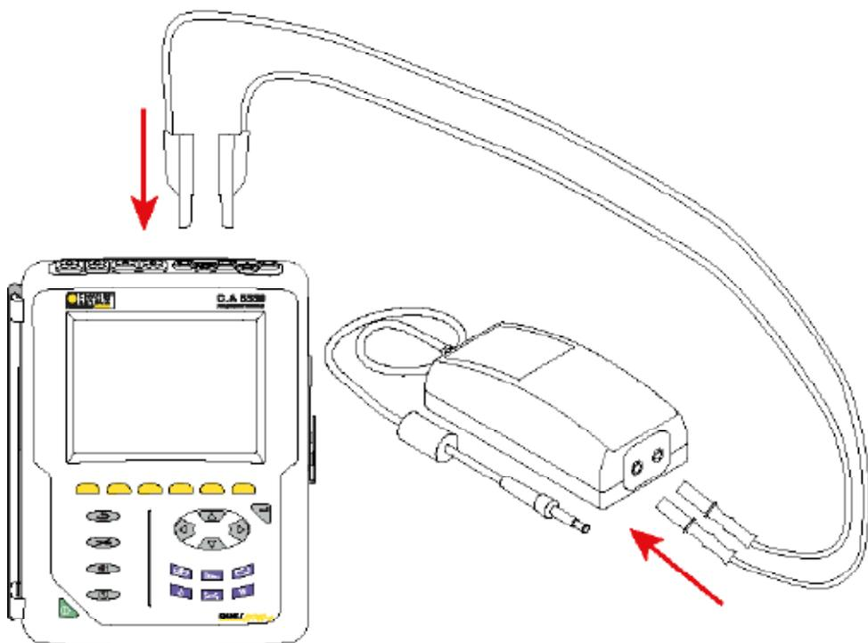
In the example above, the adapter is connected between the neutral (N) and phase L1.
