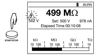
Press the **START/STOP** button again to stop the measurement.
