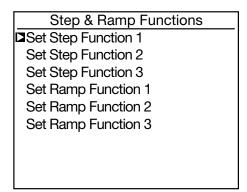
**Set Step Function 1, 2, and 3:** In the case of a measurement with a stepped voltage, used to set the voltages and the durations of the steps.
