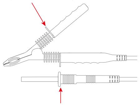
Measurements of voltages ≥1000 V on supply lines should be made using the test probes only, with the user's hands behind the hand guard on the lead.
