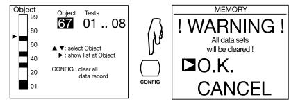
The instrument in this case completely reformats the memory, which takes a few minutes. During this time, it displays **WAIT**.
