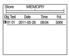
If the screen does not display the measurement and **pressing the MEM key has no effect**, press the **DISPLAY** key twice to restore the result screen, then press the **MEM** key again.
