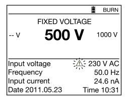
When the external voltage exceeds 25 V, the blinking (  $/! \$ ) symbol is displayed.
