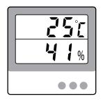
This measurement varies greatly with the temperature and the relative humidity. It is therefore essential to measure them with a separate device and to record them with the insulation value.
