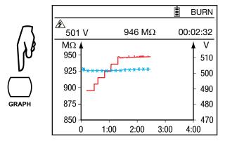
For V-VAR and V-FIXED it is also possible to change measurement parameters during the measurement, by pressing the **CONFIG** button. It is possible to fix the measurement range of the current, to add an analog filter (disturbance level low/high), or to change the test voltage if in the variable test voltage mode (V-VAR). For more details, refer to § 2.4.3.
