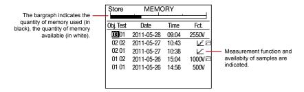
The number of measurements that can be recorded depends on the number of samples stored for each measurement.
