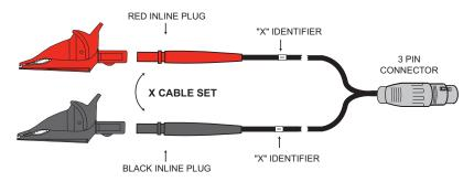
Each cable is clearly marked. The Primary (H) cable has a 5-pin connector and the Secondary (X) cable has a 3-pin connector. They cannot inadvertently be connected incorrectly.
