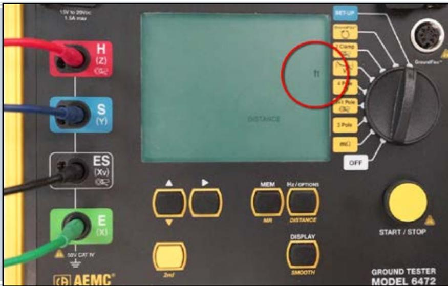
Next, turn the dial to the 4-pole  $\rho$  setting. To enter the spacing distance, press the yellow button labeled 2nd. The symbol 2nd appears on the screen, indicating buttons will now perform the actions labeled in yellow.
