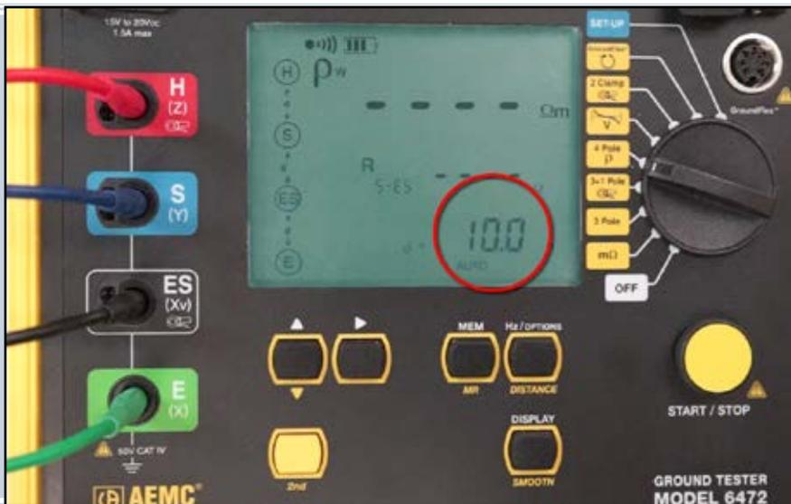
Press the DISTANCE button. The word DISTANCE appears on the screen, and the first digit in the distance field blinks, indicating it is in edit mode. Use the Up and Right buttons to navigate through this field and make selections. For example, to set the distance to 10 feet, press the Right button to navigate to the second digit and press the Up button to change this to 1. The field should now be set to 10 feet.
