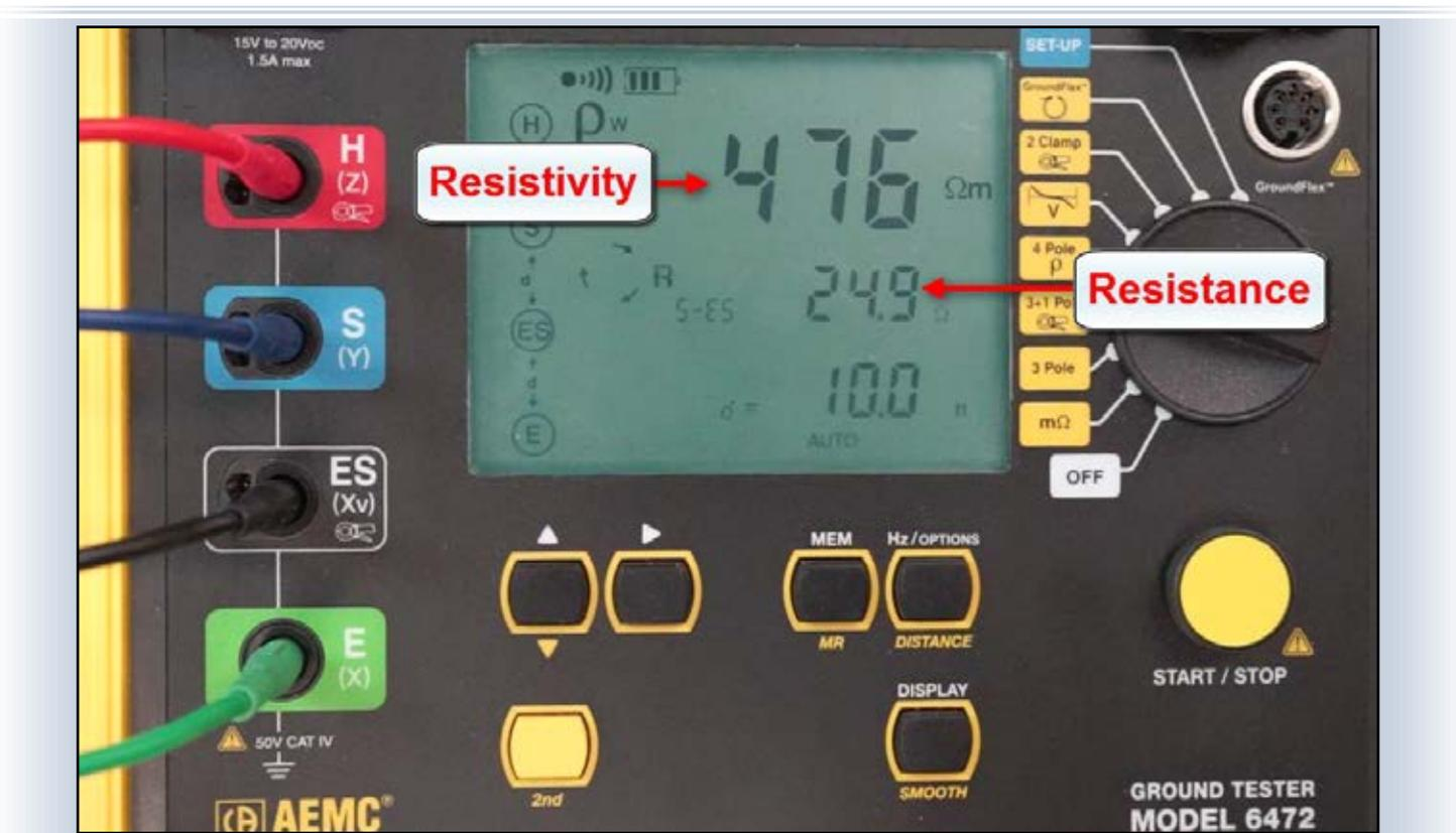
You are now ready to take a soil resistivity measurement. To do this, push the START/STOP button and hold it down for at least two seconds. After a few moments, the resistivity reading appears, displayed in ohm-meters. The resistance of the soil between the two potential electrodes is also displayed, in ohms.
