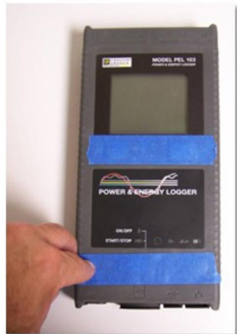
2. Tape the PEL's endplates to the back cover, as shown below. This helps ensure that the endplates remain attached to the back cover when you remove the front cover.
