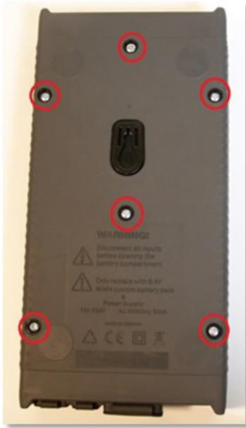
4. Using a Torx T10 screwdriver, remove these fastening screws.
