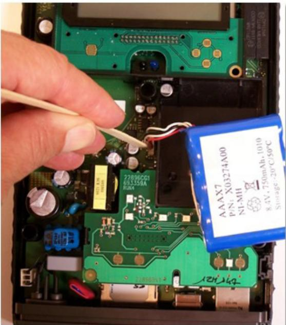
10. Place the replacement battery into the compartment provided for it within the PEL. When doing this, ensure that the battery's connector wires are positioned as shown in the illustration on the left below. Be sure the wires do not cross over the top of the post, as shown in the right illustration below. If the wires are placed over the post, they will likely be damaged when you replace the PEL top cover.
