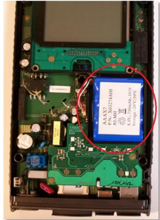
7. Gently remove and unplug the battery from the PEL. A small non-conductive implement such as a drink stirring stick (shown below) can be useful for doing this.
