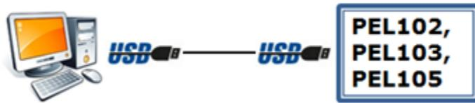
1. Connect the PEL to an available USB port on the computer using the supplied USB cable. Provided you have a “default” Windows layout with the taskbar at the bottom of the screen, a popup should appear in the lower right corner indicating that the device driver is installing.
