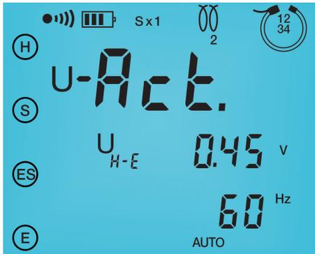
Live voltage is measured between the tower and the measurement auxiliary electrode to ensure accurate testing by verifying the electrodes distance is sufficient.
