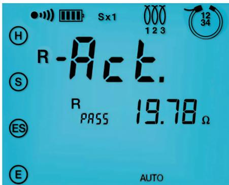
Passive resistance of the tower is calculated using leakage current and present voltage.
