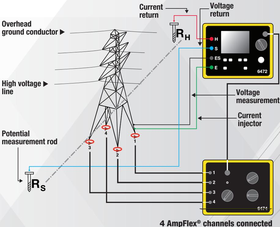
*Flexible sensors measure leakage current down tower legs*
