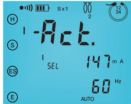
Leakage current can be displayed for each leg of the tower plus the summation of all legs together.
