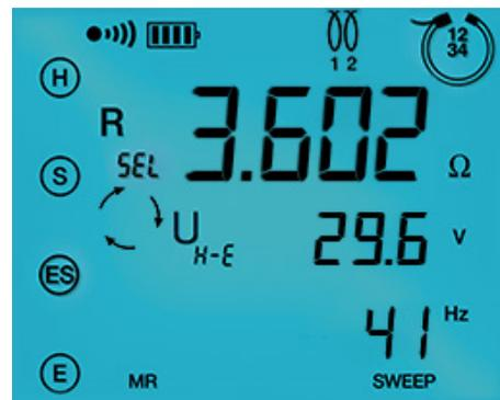
Sweep mode tests allow for multiple test frequencies to be used in succession. Data from sweep mode tests are automatically stored in the instrument and can be plotted to profile impedance values that may be incurred due to lightning.
