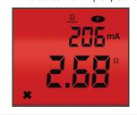
At each new measurement, the instrument indicates the difference between the new reading and the reference measurement, along with the difference in %.
