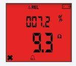
If the difference exceeds the programmed threshold, the \*symbol is displayed and the backlight turns red.
