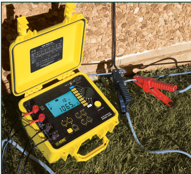
Model 6255 is a 10 A low resistance Micro-ohmmeter designed for both plant maintenance and field use. It is uniquely designed to conduct tests on bonds, contacts, joints and switches, and is an ideal device when conducting bond verification on a grounding system.
