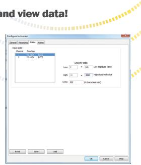
Scaling can be programmed to include lower and upper values and units for each channel
