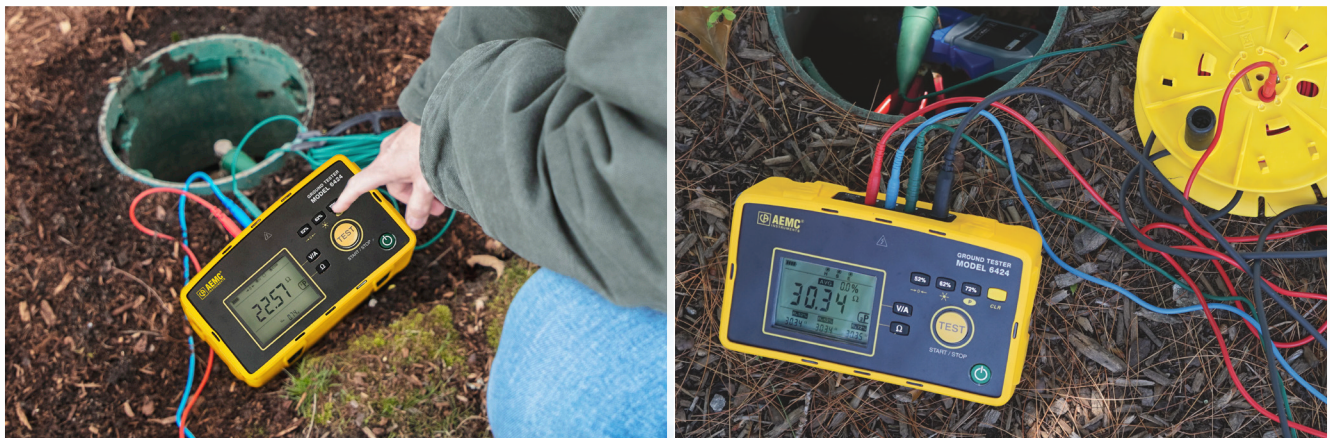
The Digital Ground Resistance Tester Model 6424 performs 2-pole resistance and 3-pole ground resistance measurements.
