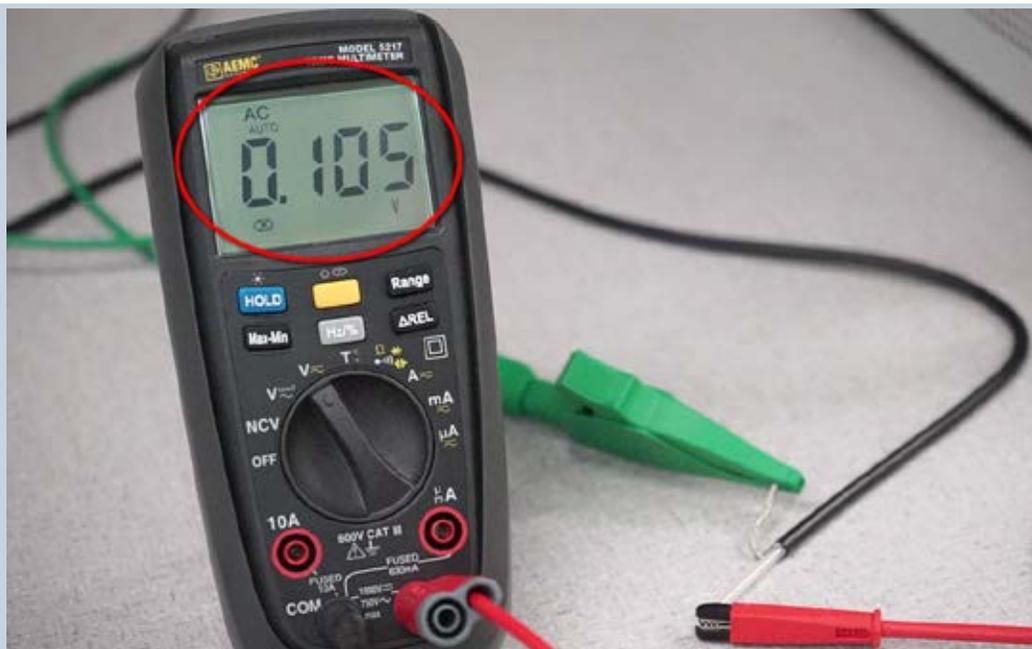
Notice that the noise voltage has dropped to around 100mV, nearly two orders of magnitude lower than our previous reading. In other words, grounding the shielding has reduced noise voltage within the cable by around 98%!
