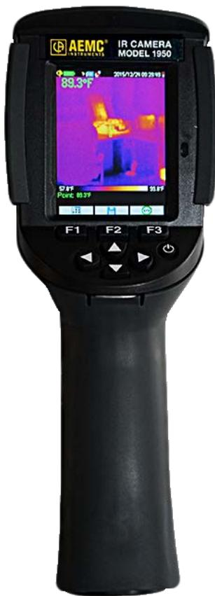
The instrument features Bluetooth for connecting to measurement instruments and a headphone for recording narration. You can download stored thermograms to a computer running CamReport software (provided with the instrument) for image processing, analysis, and report generation.
