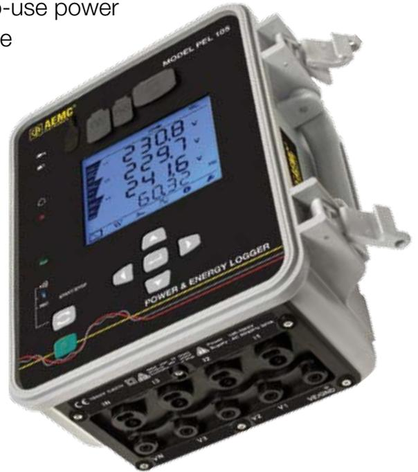
This measurement data is then used to calculate numerous values, including active, reactive, and apparent power and energy;  $\cos \phi$ ,  $\tan \Phi$ , and Power Factor (PF); crest factor, harmonics and total harmonic distortion (THD); and others. Quantities can be aggregated from 1 minute to 1 hour and stored in a SD-Card or SDHC-Card (up to 32 GB). The PEL 105 is designed for full outdoor use, resistant to both water (IP67) and sunlight (UL746C f1). The instrument
