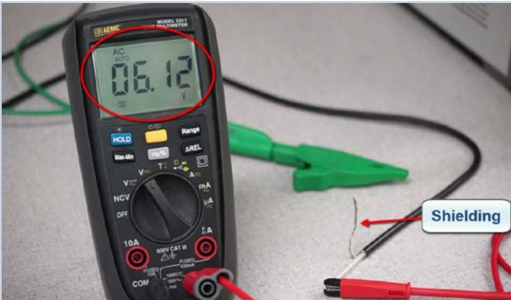
As you can see, the noise voltage being generated within the cable is over 6V, a voltage that could potentially corrupt data sent through the cable.
