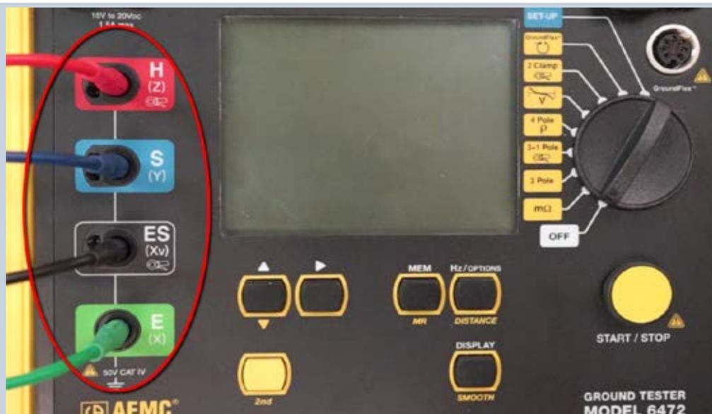
The two outer electrodes are connected to the instrument's outer terminals, labeled H and E. The inner electrodes are connected the inner terminals, labeled S and ES.
