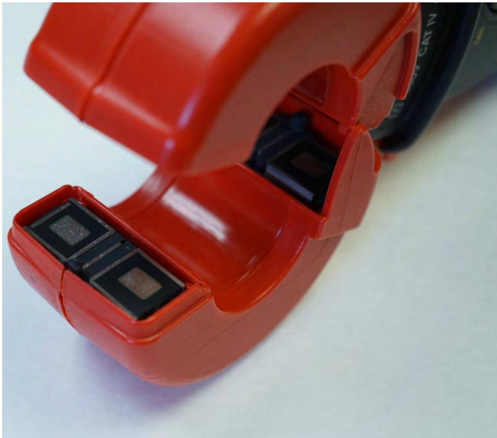
The test voltage is transmitted at a specific frequency. This allows the clamp to distinguish the induced current from other currents that may be present, such as leakage.
