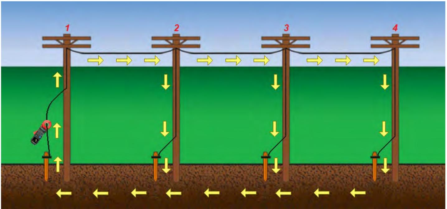
Placing the clamp around any one of the electrodes measures the resistance of the entire loop. For instance, in the preceding illustration the instrument has been clamped around electrode #1. The reading combines the resistance of #1 plus the series/parallel resistance of the group consisting of #2, #3, and #4.
