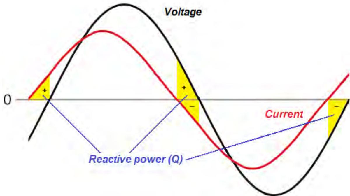
The shaded regions represent the difference between apparent power and actual power. This difference is known as *reactive power* (also called "useless power" or "watt-less" power) and is represented by the symbol  $Q$ . Reactive power is not consumed by the load; it simply "bounces" back and forth between the load and the source without being transformed into mechanical, heat, light, or other forms of energy.
