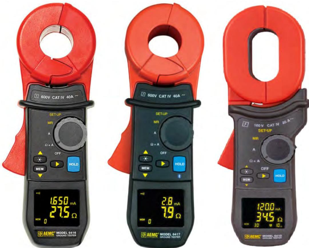
Clamp-on ground resistance testers can be used in multi-grounded systems -- simply clamp the instrument around the ground conductor or rod below all metal return paths and measure its effective grounding electrode resistance.
