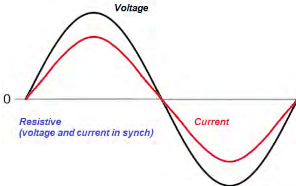
In a resistive AC network, all non-zero points in the wave yield usable power. In this case, the network's apparent power equals its actual power ( $P = S$ ), the same as in a DC circuit.
