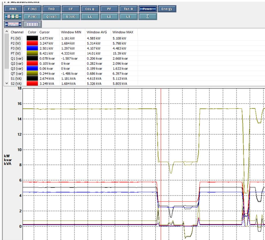
Buttons allow you to simplify the display to show only P, Q, or S values. Another button displays Power Factor for each phase and total:
