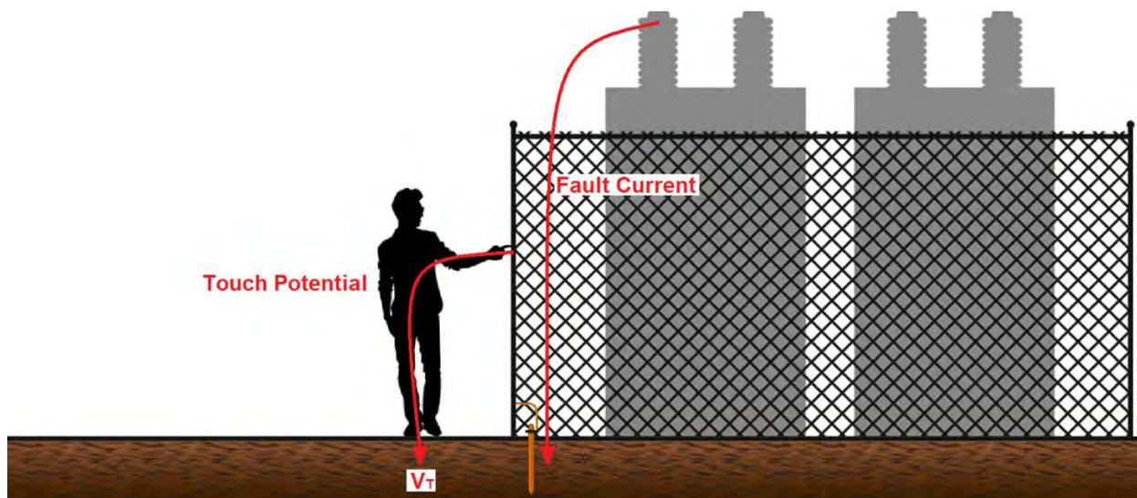
Grounding systems should be designed to ensure touch potential stays below the level that can be withstood by the human body. This includes calculating the drop of potential between a reference point (for instance the fence grounding system) and a point one meter (3.28') away, the so-called "reach distance."
