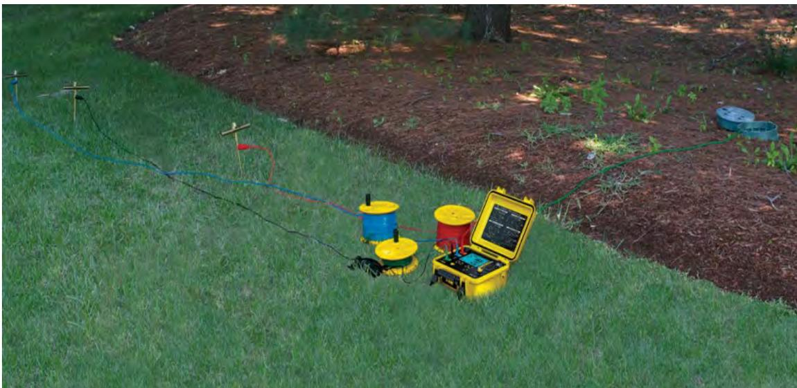
The instrument is connected to the grounding electrode system and an auxiliary electrode that injects current into the soil to simulate the fault. In between and in-line with these electrodes are placed two potential electrodes, typically one meter apart to simulate a human stride. These electrodes measure drop of potential to determine the resistance between them. This resistance and the fault current are then plugged into the Ohm's Law formula to calculate step potential ( $V_s$ ).
