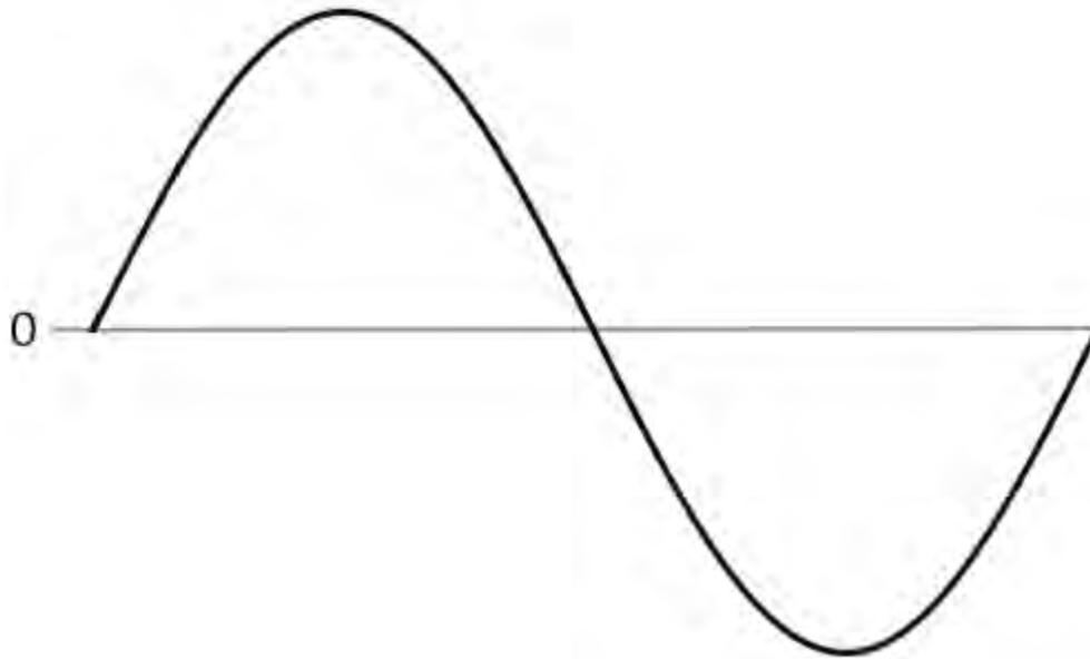
For "clean" AC power undistorted by factors such as harmonics, the sine wave is perfectly symmetrical and spends as much time above zero as below it.
