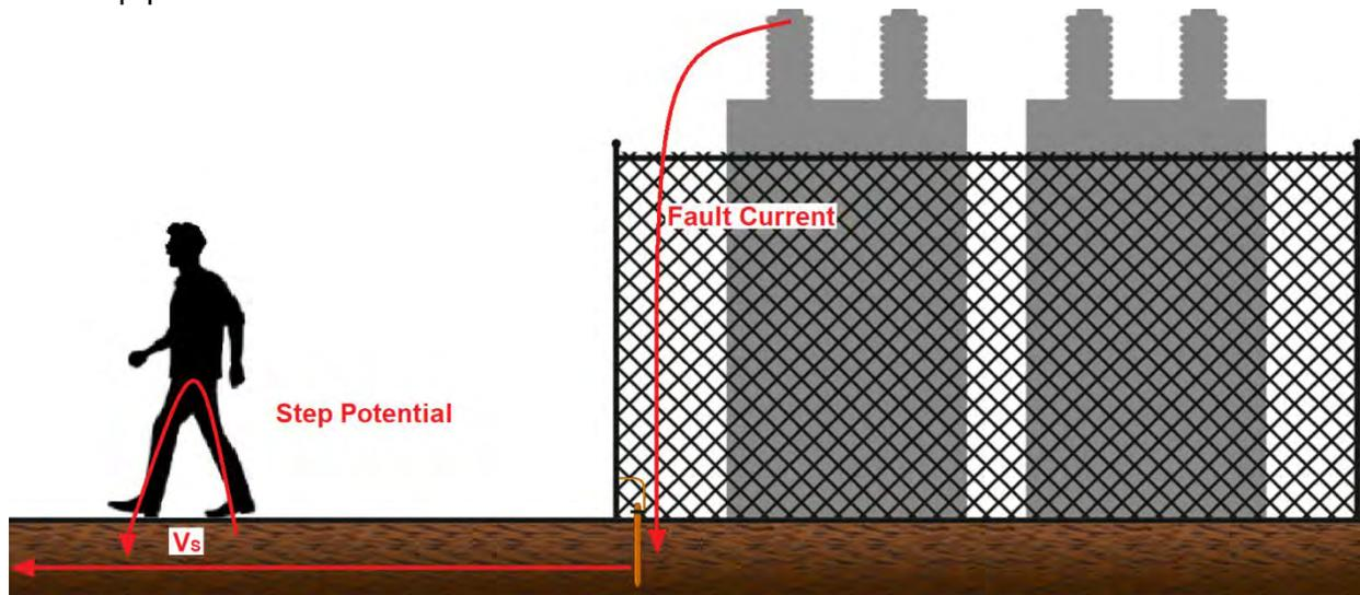
Depending on conditions, dangerous step potential can exist a significant distance from the grounding system. Factors include the amount of fault current that enters the ground, along with soil resistivity – the higher the soil resistivity, the higher the step potential.
