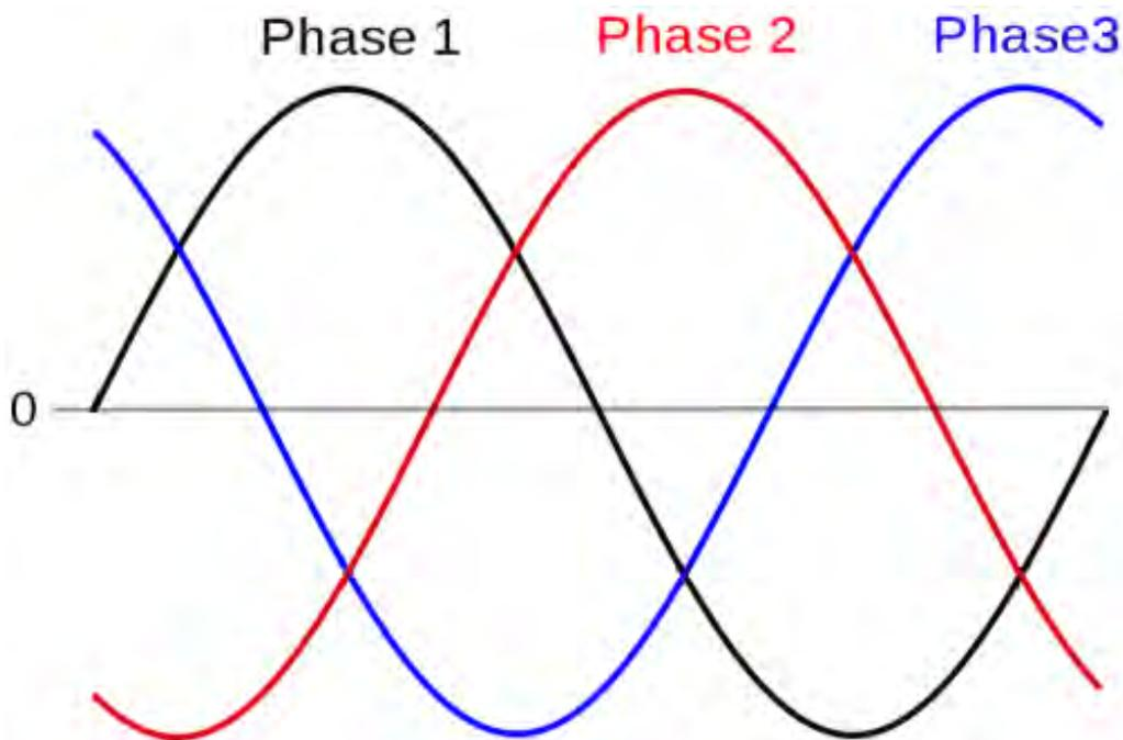
Each wave represents electricity periodically oscillating between its positive and negative values.
