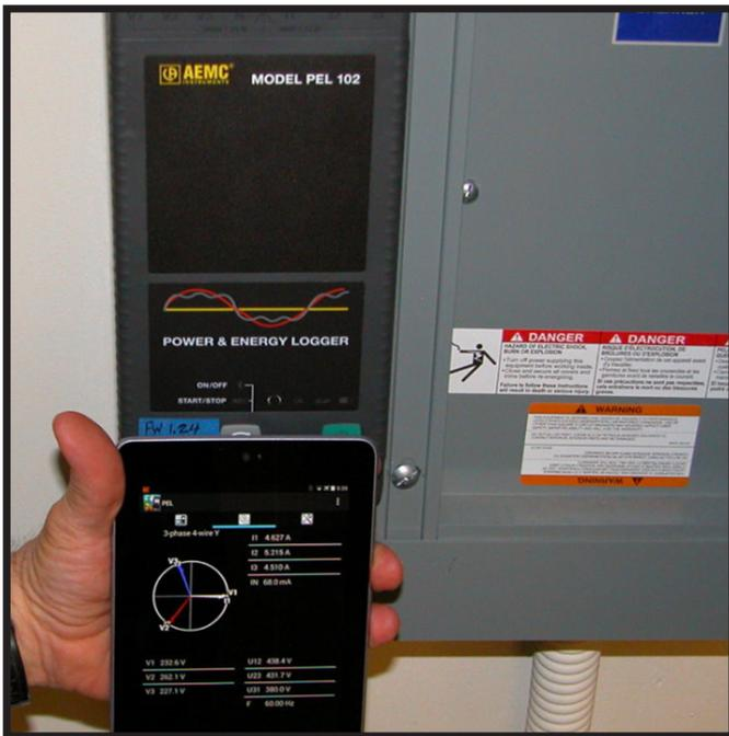
*Power & Energy Logger app running on an Android device, with a PEL 102 in the background*
