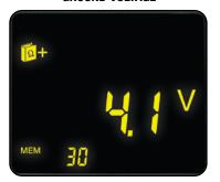
Indicates voltage potential at the point of measurement
