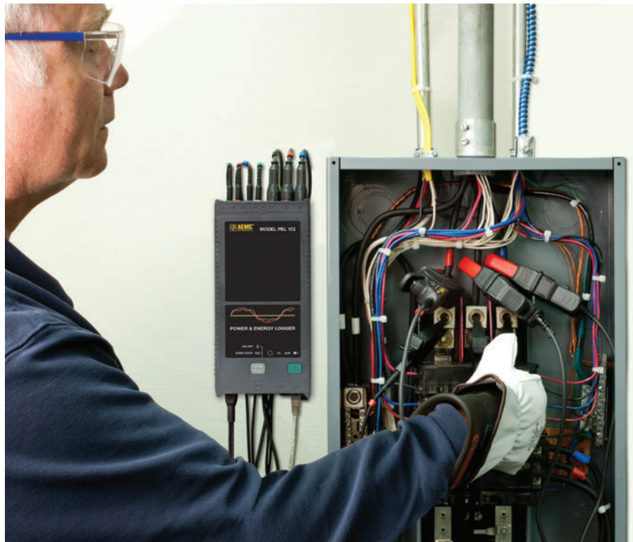
(Figure 1) Easily connect current sensors and voltage leads without power interruption.
