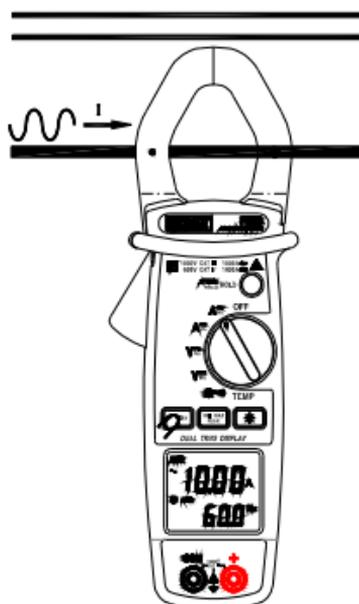
Position the switch on  $A_{\tilde{}}$ , and press the **DISPLAY** key.
