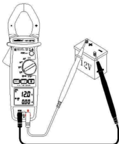
Connect the red test lead to the "+" terminal and the black test lead to the "COM" terminal.
