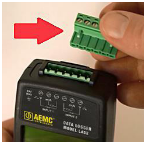
Figure 23. Terminal strip (upper right)
