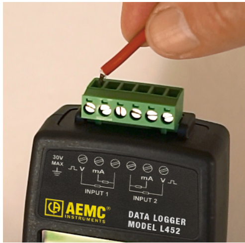
Figure 24. Inserting a lead into the terminal strip
