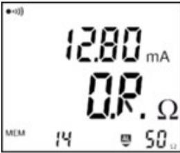
When the impedance measurement is  $> 1200 \Omega$ , the instrument displays **OR**.
