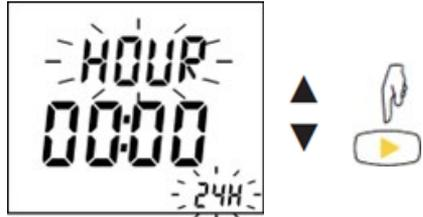
Confirm by pressing ►. The hours reading blinks. Set it using ▲ and ▼ and confirm by pressing ►.
