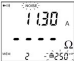
When the current exceeds 10 A, the impedance measurement is not displayed (dashes appear in the measurement field).
