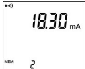
When the measurement has stabilized, you can press the **HOLD** key to freeze it and/or **MEM** to record it in memory. You can also use the **AUTO-HOLD** function (see § 3.4) to freeze the measurement automatically when the clamp jaws are opened. This can be useful when you have only one hand free to make a measurement. To facilitate making measurements, you can configure an alarm on the current measurement value (see § 3.4).
