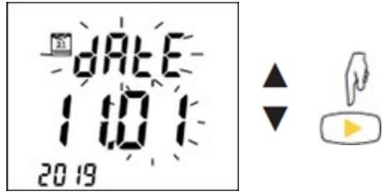
Press ►. The date blinks; set it using ▲ and ▼ and confirm by pressing ►.
