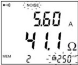
Display of the **NOISE** symbol during the impedance measurement indicates that the current ( $> 5\text{ A}$ ) or voltage ( $Z \times I > 25\text{ V}$ ) is too high, making the accuracy of the displayed measurement uncertain.
