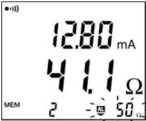
The alarm indicator on the display blinks and the instrument emits a continuous audible signal.
