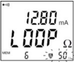
When the impedance measurement is  $< 1 \Omega$ , the display alternately indicates the measured value and **LOOP**, indicating the value is very low for a valid ground impedance measurement and most likely indicates the measurement is through a wire loop rather than through the earth.
