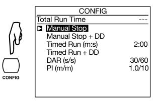
Use the ▲ ▼ arrow buttons to select Manual Stop + DD or Timed Run + DD (manual or automatic measurement).
