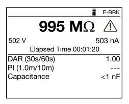
The **DISPLAY** button is used to look up all information available after the measurement. This information depends on the type of measurement chosen (see § 2.4.4).
