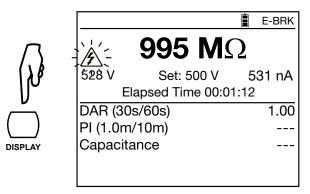
In the case of a step test voltage (10 steps at most) or ramp test voltage (3 steps), the progress of the steps will be indicated.
