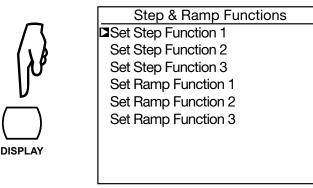
Set Step Function 1, 2, and 3: In the case of a measurement with a stepped voltage, used to set the voltages and the durations of the steps.
