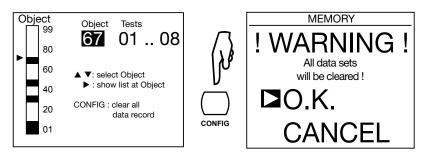
The instrument in this case completely reformats the memory, which takes a few minutes. During this time, it displays **WAIT**.
