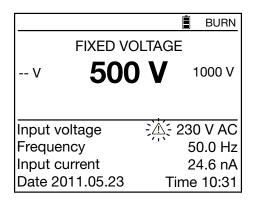
When the external voltage exceeds 25 V, the blinking ( 1) symbol is displayed.
