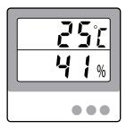
This measurement varies greatly with the temperature and the relative humidity. It is therefore essential to measure them with a separate device and to record them with the insulation value.
