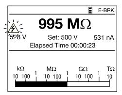
If the measurement is unstable, it is possible to apply a digital filter by pressing the **FILTER** button.
