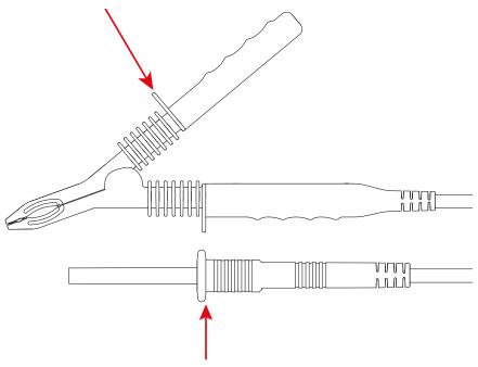
Measurements of voltages  $\geq$ 1000 V on supply lines should be made using the test probes only, with the user's hands behind the hand guard on the lead.
