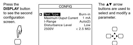
The second configuration screen depends on the rotary switch setting.
