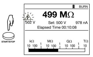
Press the **START/STOP** button again to stop the measurement.
