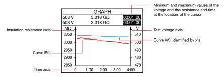
This curve is plotted using samples recorded during the measurement.
