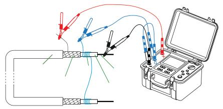
Using the guard eliminates the influence of the surface leakage current. A conducting wire must be wrapped around the insulation.
