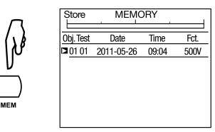
If the screen does not display the measurement and **pressing the MEM key has no effect**, press the **DISPLAY** key twice to restore the result screen, then press the **MEM** key again.
