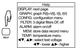
A long press on the **HELP** button (>2 s) allows setting of the display contrast and the backlighting (see § 3.1).
