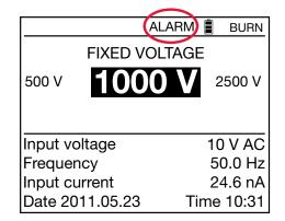
The ALARM symbol is displayed if the alarm is enabled.
