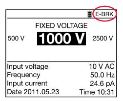
Stopping the test at a preset current (Break at I-limit)
