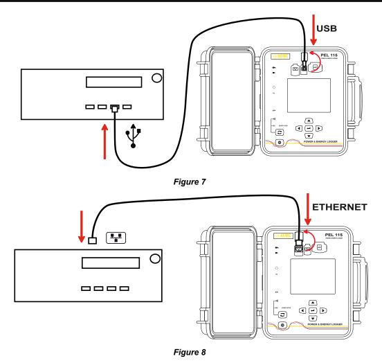
Then, for whichever link was chosen, open the PEL Control Panel (see § 6) to connect the instrument to the PC.
