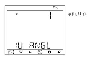
Phase angle between line current and phase voltage
