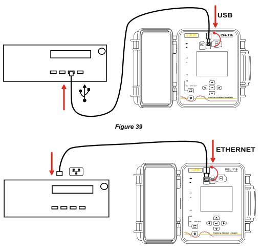
Then, whichever link was chosen, open the PEL Control Panel to connect the instrument to the PC.
