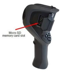
Camera files (images, audio, and setup) are stored in the micro SD memory card located on the left side of the head (see photo below). If this card is not installed, an error message appears when the camera attempts to access it. This card is provided with the camera.
