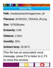
A vocal message is played back using the Bluetooth headset, which must be connected to the camera (see § 7.2.1).
