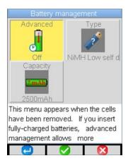
The Battery management menu appears when the batteries have been removed. If you insert fully-charged batteries, advanced management allows more options.
