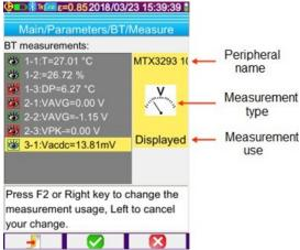
This menu displays measurements received from the connected devices during the last acquisition.
