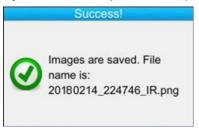
If acquisition is stopped, each additional press of the trigger creates a new **derived** image (same date of acquisition), differentiated by an index letter added to its name (see § 5.1).
