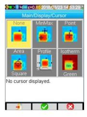
Below the image is the Measurements display area (see § 2.3.1.3). The displayed data depends on the measurement cursor setting. By default, no measurement cursor is selected, resulting in no measurement data displayed in the screen. To change the cursor setting:
