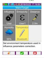
The measurements replace the user data entered in the Target menu (shown to the left), provided that the Influence setting is User (see § 4.2.2).
