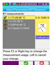
You can use a measurement from a connected device as an **influence** to compensate for an environmental factor. The measurement will be used to calculate the amount of correction that needs to be applied. Note that this option is available only for temperature, humidity, and distance measurements.
