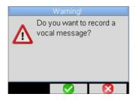
You can create a vocal message for the image. This requires a Bluetooth headset connected to the camera (see § 7.2.1). The recording can be up to 30 seconds long. The vocal message can be added only after you have created the image file. After the message appears displaying the name of the new file, if the headset is connected another message prompts you to record a vocal message (as shown to the left).
